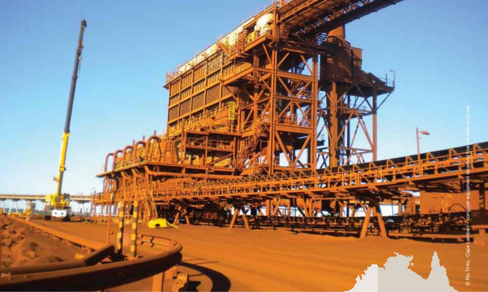
© Rio Tinto. Cape Lambert – conveyor equipment recycling fine ore from lump ore.
